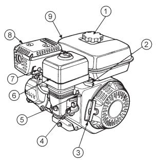
Figure 4. Engine Controls and Components (Honda GX390K1QWT2)
